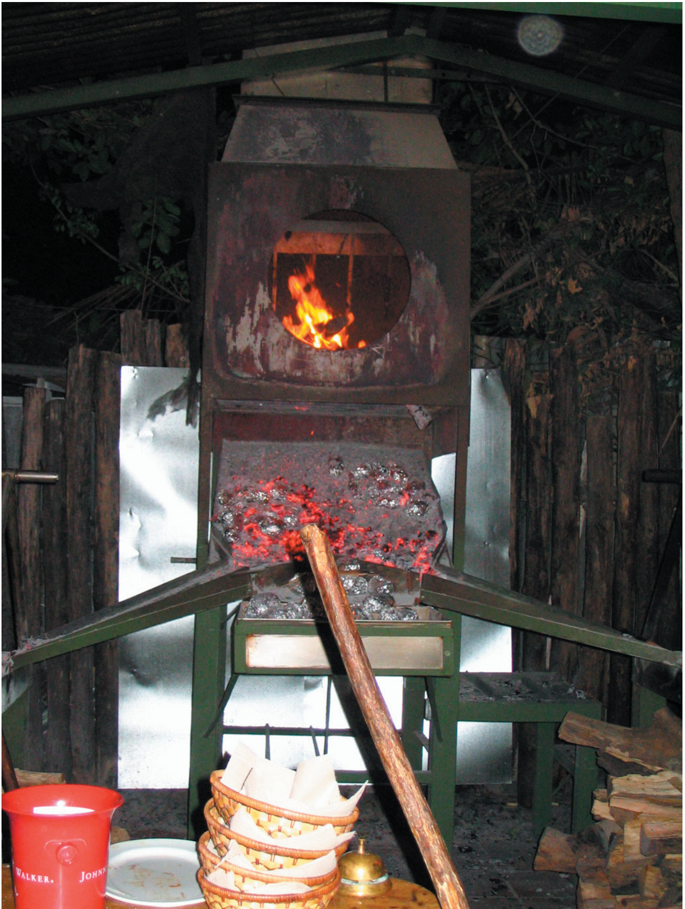
The Heart of La Guarta restaurant. This massive furnace was continuously stoked with palm wood. The resulting coals are shoveled down the gutters to either side into large basins over which meat and vegetables are grilled.
